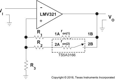
Figure 24. Gain-Control Circuit for Operational Amplifier
