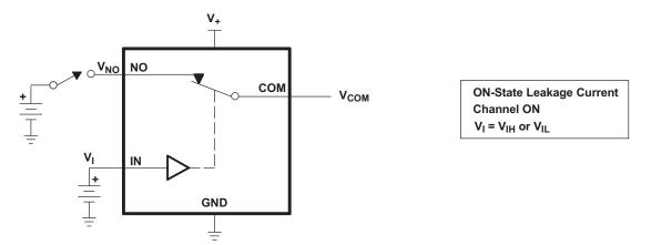
Figure 15. ON-State Leakage Current (I<sub>COM(ON)</sub>, I<sub>NO(ON)</sub>)
