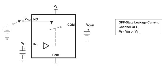
Figure 14. OFF-State Leakage Current (I<sub>COM(OFF)</sub>, I<sub>NO(OFF)</sub>, I<sub>COM(PWROFF)</sub>, I<sub>NO(PWR(FF)</sub>)
