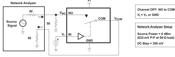
Figure 19. OFF Isolation (O<sub>ISO</sub>)
